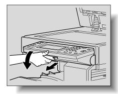
The angle of the control panel stops at the middle position.
